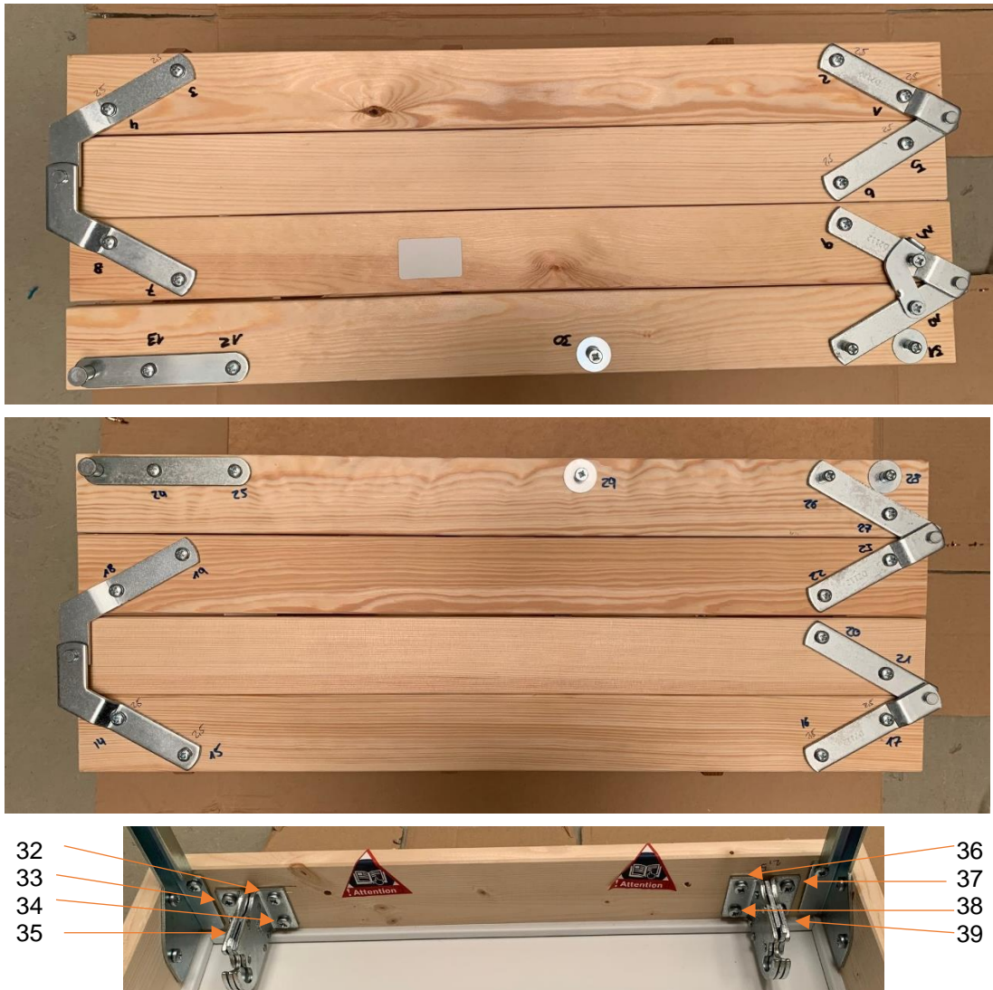
Figure 42: Overview of the tested screwed joints
