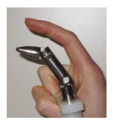
Housing of machines as well as products, such as fans, must be designed in such a way that a worker's finger does not come into contact with dangerous mechanical or electrical parts. This is tested with a standardised test finger, which is modelled like a human finger.
